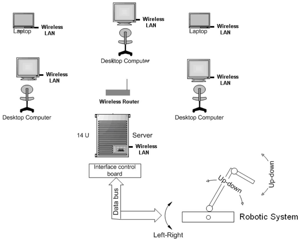
**Fig. (2) The same Robotic system remotely connected through wireless LAN.**
