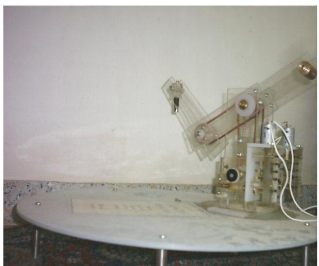
**Fig. (6) Three-joint Robotic system in different movements.**
