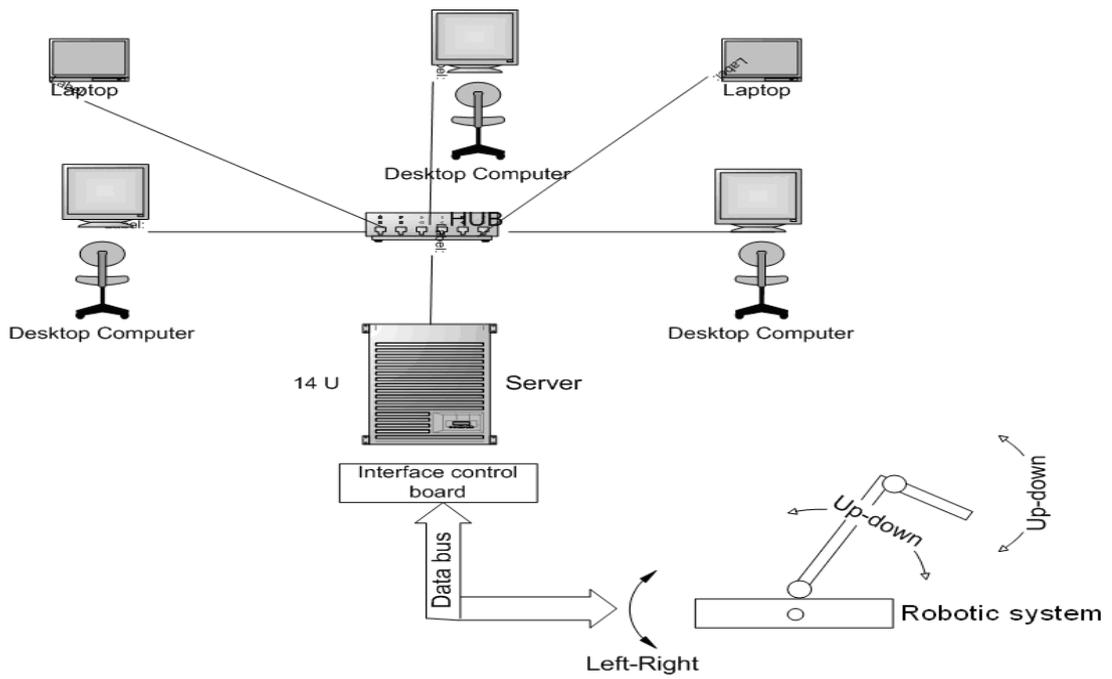
**Fig. (1) Robotic system remotely connected through LAN.**
