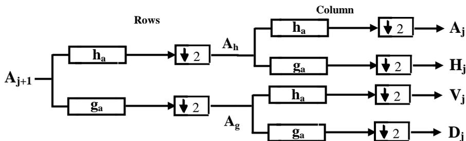
Figure (3) one stage of analysis 2D-DWT stage
