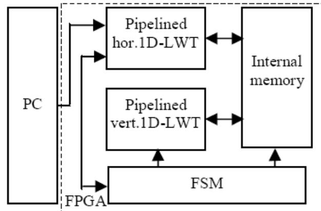
Figure (1) : block diagram of proposed structure
