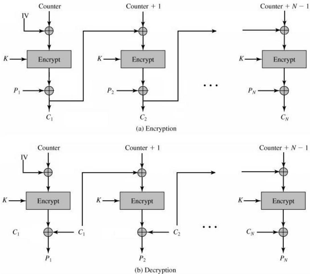
**Fig.2: Counter Cipher Block Chaining (CCBC) Mode**
