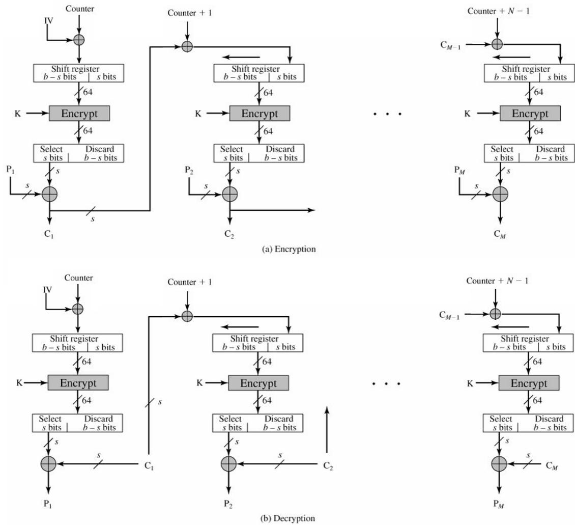
**Fig.3: s-bit Counter Cipher Feedback (CCFB) Mode**
